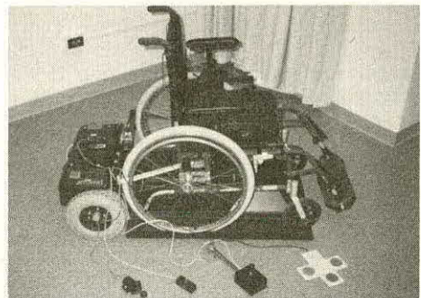
Photo 2: Powered Wheelchair Mobility Simulator mounted with manual wheelchair. Also, switch control options are shown.
